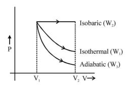
W = Area under P-V curve  $\Rightarrow$  W<sub>2</sub> > W<sub>1</sub> > W<sub>3</sub>
